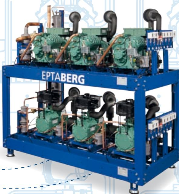
EptaBerg was designed to simplify handling, using both forklift trucks and cranes, and installation. If necessary, the two-level model can be dismounted and reassembled directly in plant room.
